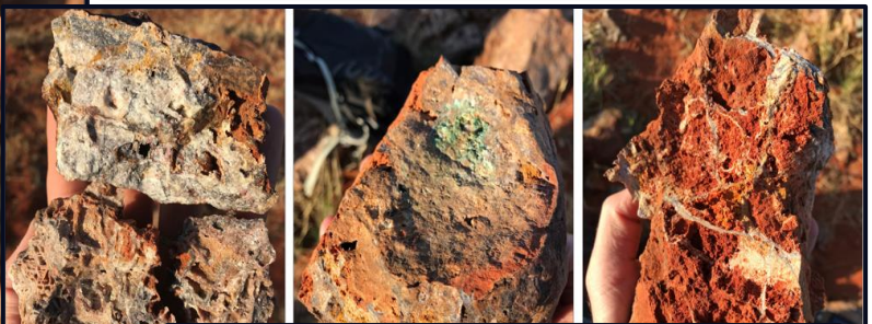
Mineralised stockwork (>0.5% Cu) in granite at the Sunset Boulevard Prospect along strike from Ningaloo at the Camel Creek target
