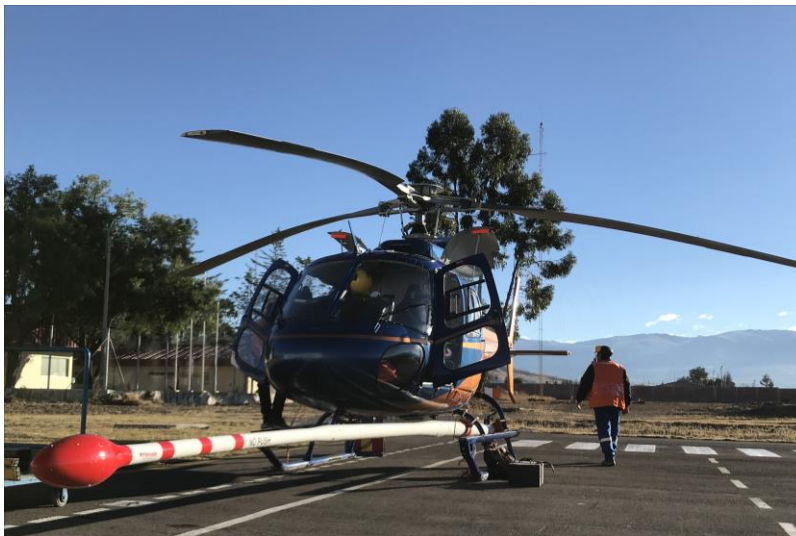
Figure 1 LEFT: The helicopter involved in the survey (pictured here) was based out of Huamanga Province capital Ayacucho, which is a short flight southeast of the Greater Riqueza Project. The distinctive tool extending from the front of the helicopter is a KMAG4 magnetometer counter.
