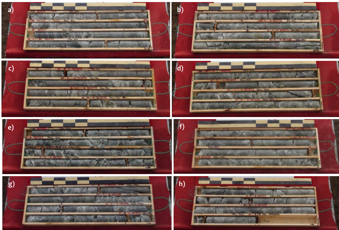
Figure 2: Core box photos of CH-DDH002: a) 68m to 72m; b) 80m to 84m; c) 91m to 95m; d) 102m to 106m; e) 113m to 117m; f) 124m to 128m; g) 136m to 140m; and h) 147m to 150m (EOH). The geology is described as being a hydrothermal breccia, logged from the surface to 150m.
