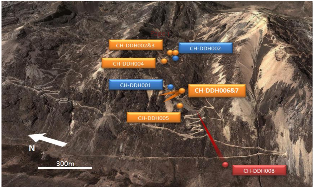
Figure 2: 3D terrain image of the Chanape Project area looking towards the ENE. CH-DDH006 & 7 are twinned holes drilled across Hydrothermal Breccia 8. Also shown is the position and rough projection of the current deep hole (CH-DDH008). This hole is testing porphyry “into the page” (represented by a diminishing triangle). The image also shows the extent of existing access tracks across the project area.
