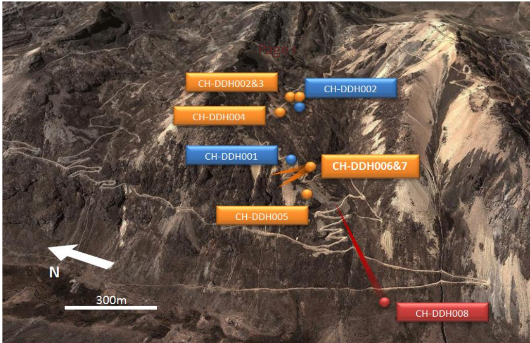
Figure 1a: 3D terrain image of the Chanape Project area looking towards the ENE. Drill hole CH-DDH008 is positioned SW of CH-DDH001. This hole tested the possible south west extension of the known porphyry in CH-DDH001.
