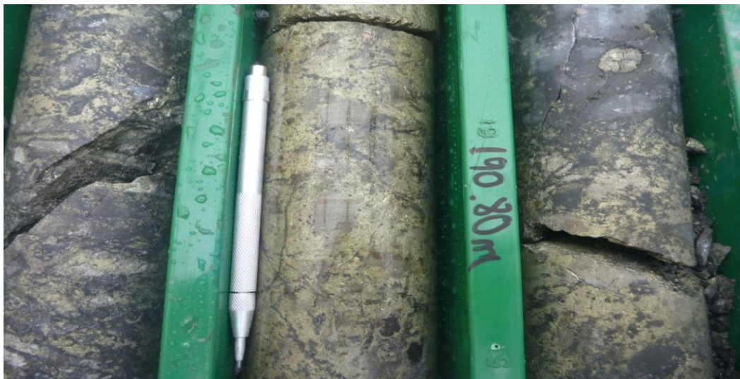
Figure 1: Massive visible chalcopyrite at 190.8m in CH-DDH012. Assay results of 190m-191m returned 13.4% Cu, 0.031% Mo, 1.4g/t Au and 186g/t Ag .
