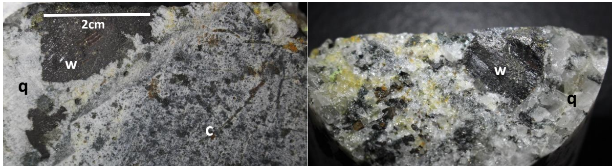
Figure 1: Wolframite at 59.3m within the upper hydrothermal breccia in CH-DDH012. LEFT: Cut core surface showing large wolframite crystal (w) in qtz matrix (q) adjacent to altered breccia clast (c): RIGHT: Broken core surface showing same wolframite crystal.
