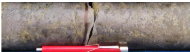
Figure 3 LEFT: Core photo at 288.0m in CH-DDH019. The grade of the corresponding 288-289m sample is >10.0g/t Au, 23.1g/t Ag, 0.24% Cu and 0.23% Pb. Two samples between 288m and 290m are greater than detection limit of 10g/t Au.
