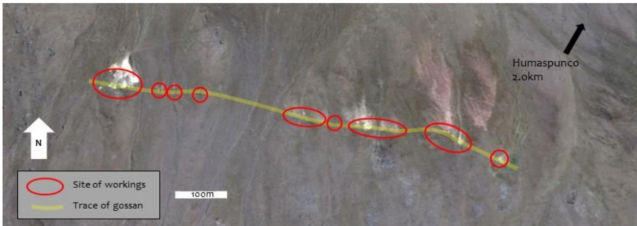
Figure 5: ABOVE Plan showing the projected EW 750m trace of the Uchpanga structure zone. The old Rita Maria workings are located at the far western end, with the dump material (white scree) clearly visible.
