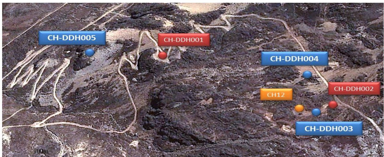
Figure 1: Location plan of Inca’s drill holes at Chanape. BLUE: Recently completed holes by Inca. RED: Inca’s Q1 2013 holes including the “discovery” hole CH-DDH001, which intersected mineralised porphyry. ORANGE: Drill hole completed by a previous explorer.
