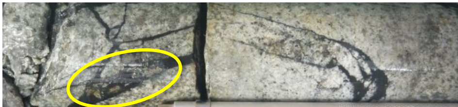
Figure 2: CH-DDH012 at 508m: The monzonite is intensely altered with tourmaline/sulphide veining causing local brecciation. Sulphides associated with tourmaline are circled.
