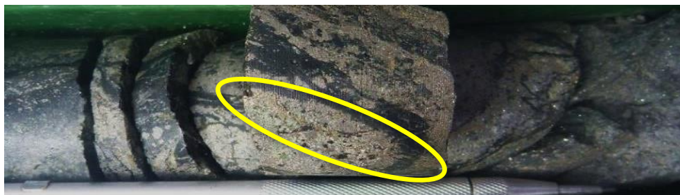
Figure 1b) CH-DDH012 at 517m: Intense brecciation of phyllic-altered monzonite with tourmaline and sulphides at 517m. As is the case in Figure 1a) the tourmaline and sulphides are closely associated. Banded fine-grained disseminated sulphides with sericite are circled.
