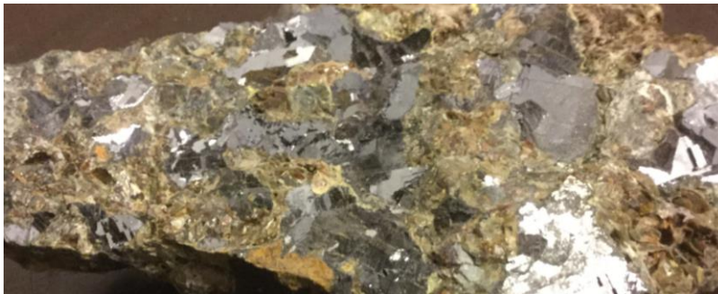
Figure 1: Vein material sampled during the current mapping and sampling programme. It contains coarse galena and fine sphalerite within a calcite-barite matrix.
