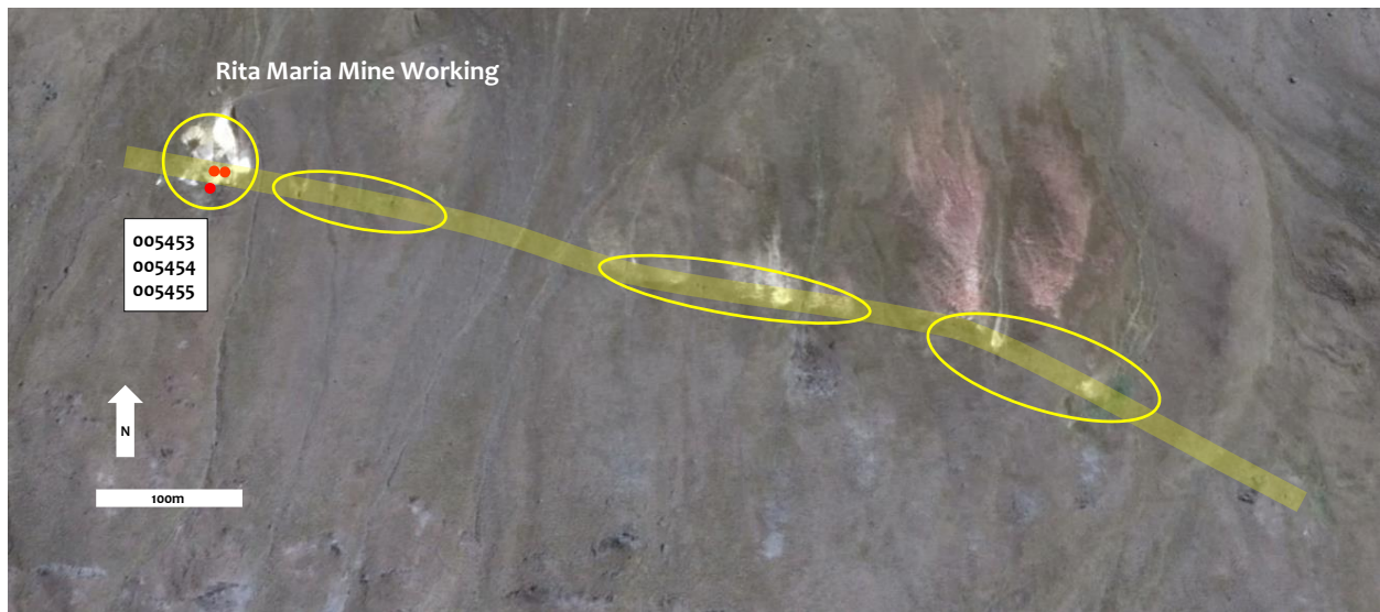
Figure 5: ABOVE Satellite image of the Uchpanga Prospect, showing the sample locations and rough trace of the gossan (transparent yellow line) and location of the workings (circled). The Rita Maria mine working is the largest in the chain of workings. It is probable the gossan is the surface representation of the vein that was mined between the 1950's to 1980's.
